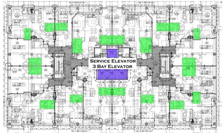
New floor layout with elevators in blue and restrooms in green.
