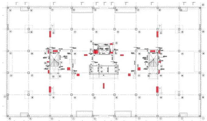
New slab cut locations for ductwork only. All plumbing fixtures require penetration.
